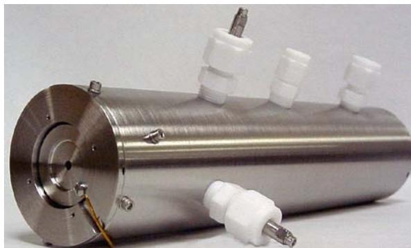
**Figure 2:** Hexapole Collision Cell with Entrance Lens
