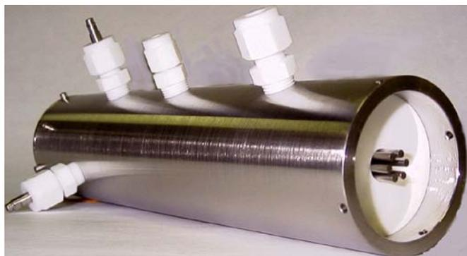
**Figure 1** Hexapole Collision Cell with Entrance Lens Removed
