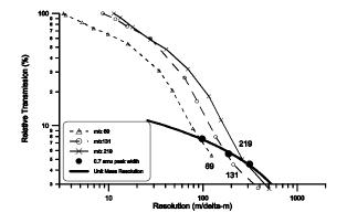
Figure 3 Relative transmission curves for 9.5 mm quadrupole (grounded entrance lens).
