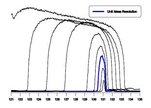
Figure 1 Transmission of m/z 131 as a function of resolution (19mm quadrupole, mass programmed entrance lens).
