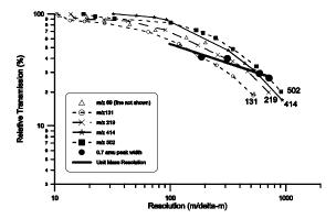
Figure. 6 Relative transmission curves for 19 mm quadrupole (mass programmed entrance lens).
