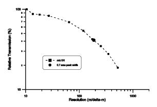
Figure 2 Relative transmission curve for m/z 131 (19mm quadrupole, mass programmed entrance lens).
