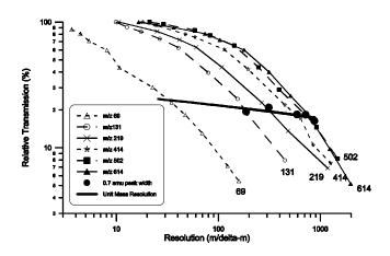
Figure 4 Relative transmission curves for 9.5 mm quadrupole (mass programmed entrance lens).
