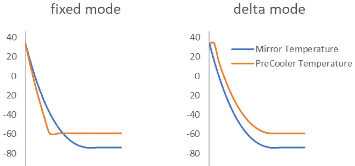
The delta mode is suitable in general, a delta of  $10\text{ }^{\circ}\text{C}$  is a good starting value most of the time. Fixed mode shall be used when fluctuations of the sample gas humidity lead to noisy precooler setpoint in delta mode or when a specific sample gas humidity should be checked.
