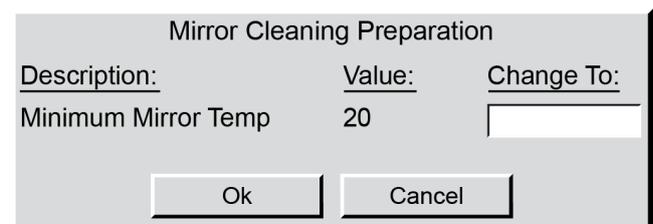
4. Enter the temperature in degrees C which the mirror must warm to during the Mirror Cleaning mode. It is recommended that you enter your current ambient temperature or higher.
