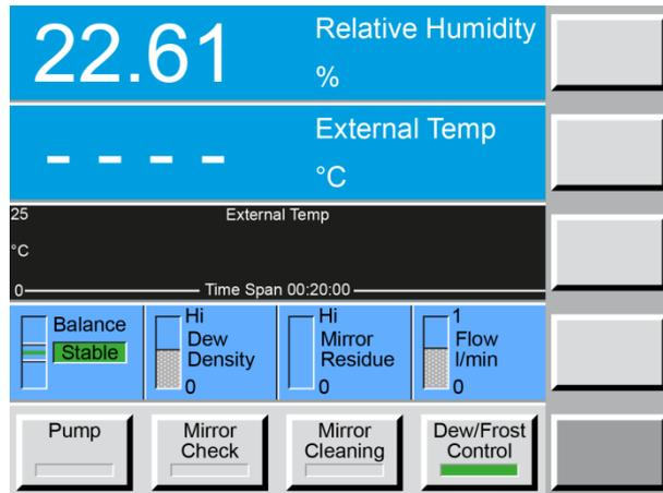
Enter the desired temperature in degrees Celsius (21 °C in this example) and activate the **Use Fixed Ext Temp** option by touching the button. When the indicator square turns green, the fixed external temperature is active.
