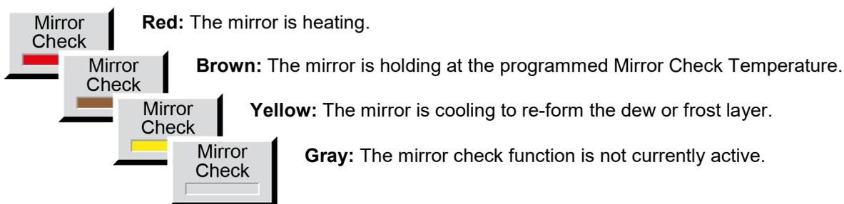
Once the system has re-established a dew or frost layer and become stable, the mirror check function is completed and the color indicator turns gray.
