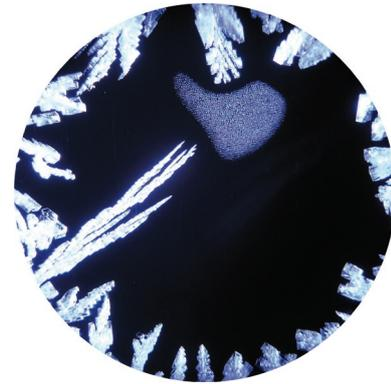
Therefore, the phase of the condensate must be known in order to avoid significant errors and to correctly calculate all humidity values, including vapor pressure, dew point, %RH, volume ratio, weight ratio, absolute humidity and specific humidity.
