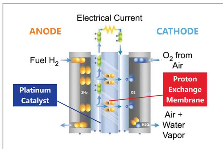
Fig. 1 Schematic and principle of operation of a PEM fuel cell
