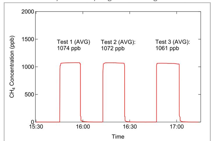
Fig. 3 Repeatability test with a ~1 ppm CH<sub>4</sub> in H<sub>2</sub> sample using a Prismatic 2 CRDS analyzer
