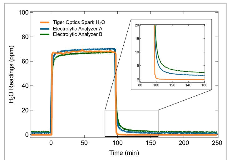
Fig. 3 Comparison of speed of response to a 67 ppm H<sub>2</sub>O intrusion. The insert shows an expanded view of the dry-down section.
