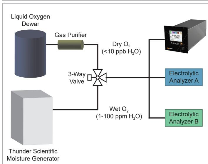
Fig. 1 Test setup for Spark H<sub>2</sub>O validation for use with medical oxygen.
