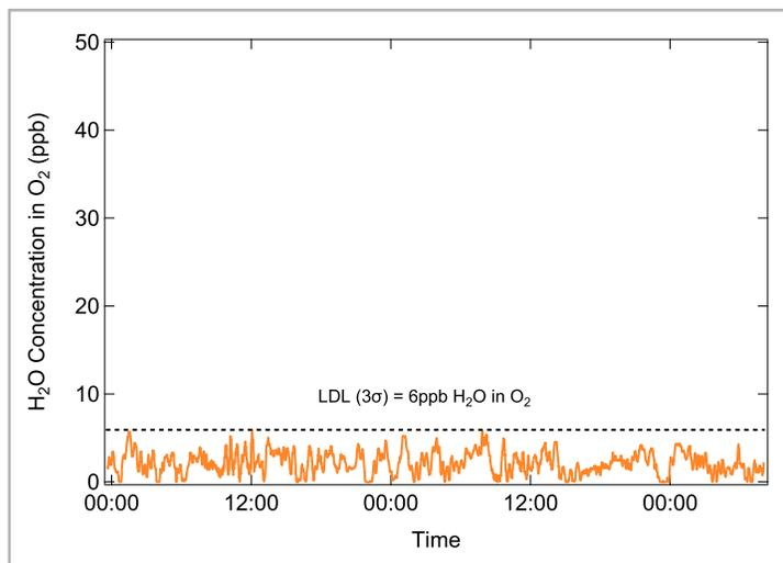
Fig. 4 Spark H<sub>2</sub>O baseline in pure oxygen over >2 days, showing consistent readings below the specified LDL.
