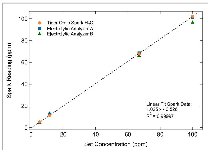
Fig. 2 Linearity comparison with values from Table 2. The linear fit of the Spark data shows an excellent linearity factor (R<sup>2</sup>) of 0.99997.
