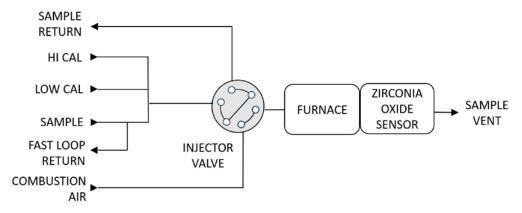
The majority of the sample gas will return to the process gas stream through the fast loop so there is no hazardous hydrocarbon emission. Only the small amount of sample gas and air mixture is completely burned in the combustion process resulting in extremely low, non-hazardous (CO<sub>2</sub>) emissions.
