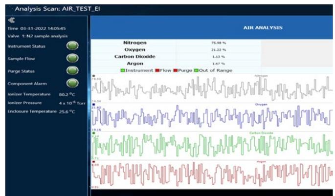
Simultaneously view current results and calculations, trends, and current analyzer status parameters with the easy-to-use Questor5 software and graphical user interface.
