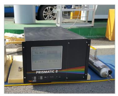
Fig. 2 Prismatic 2 at a hydrogen fueling station in South Korea (picture courtesy of Sunwoo Engineering)
