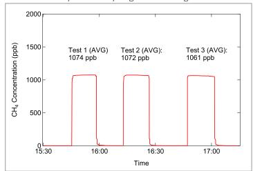
Fig. 3 Repeatability test with a ~1 ppm CH<sub>4</sub> in H<sub>2</sub> sample using a Prismatic-series CRDS analyzer
