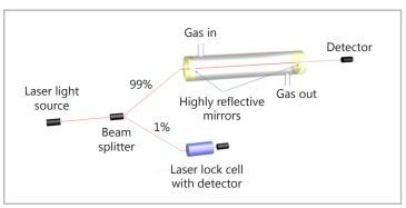
Fig. 4 Principle of Cavity Ring-Down Spectroscopy
