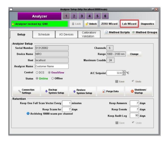
3) The Setup tab of the Lab wizard allows for the general scope or data-set of the on-demand scans to be defined. A user with Technician level privileges can only select a previously defined data-set from the drop down list. A user with Engineer level privileges can select an existing data-set or create a new data-set by clicking the **plus** button.
