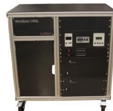
High Resolution Mass Spectrometer for Isotopic Analysis VeraSpec HRQ™
