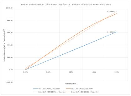
Figure 13. Dilution Curve from Helium-Deuterium Detection Limit Experiment.
