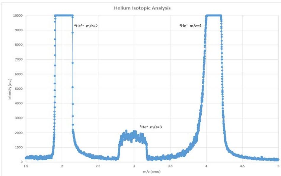
**Figure 7.** UHP Helium Scan for Analysis of  $^3\text{He}$  Isotope (1.4ppm Relative Abundance). The Resolution Was Set Appropriately for the Isotopic Analysis (Less than the Maximum Resolution for the Scan).
