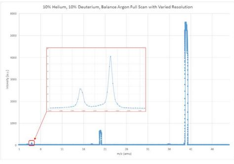
Figure 6. A Mass Spectrum of 1 – 50 amu Showing a Variable Resolution. Sample consists of 10% Helium, 10% Deuterium, and Balanced Argon.
