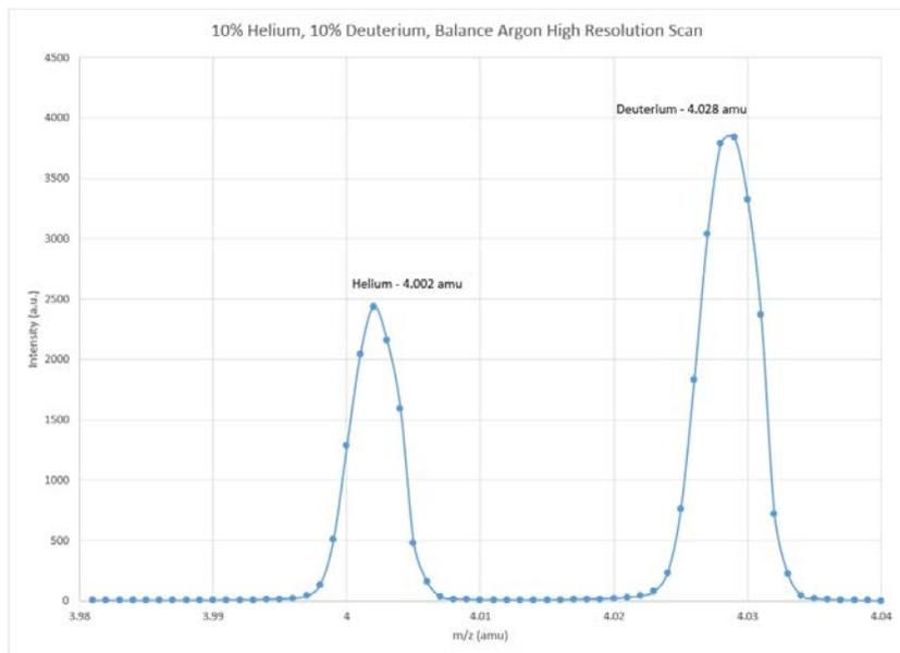
Figure 3. 3.98 – 4.04 amu Scan of 10% Helium, 10% Deuterium, Balance Argon.
