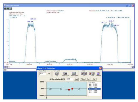
Figure 5. Resolution Calibration – Adjusted Table.
