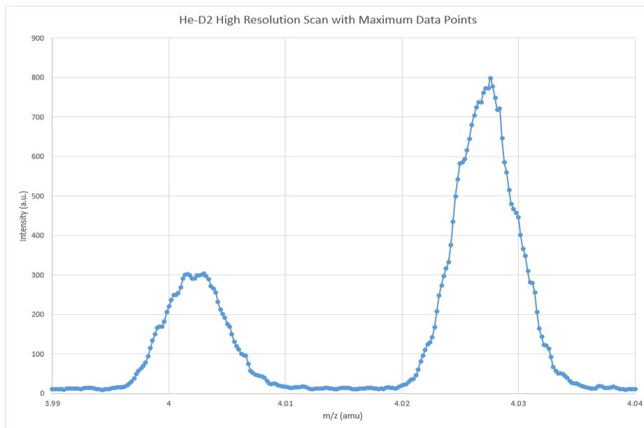
**Figure 9.** High Resolution Scan of Helium and Deuterium with Maximum Data Points (points/amu) Collected Using One Second Scan with the Maximum Amount of Points/amu. The Scan Range of  $m/z$  3.99 – 4.04 Resulted in 250 Data Points.
