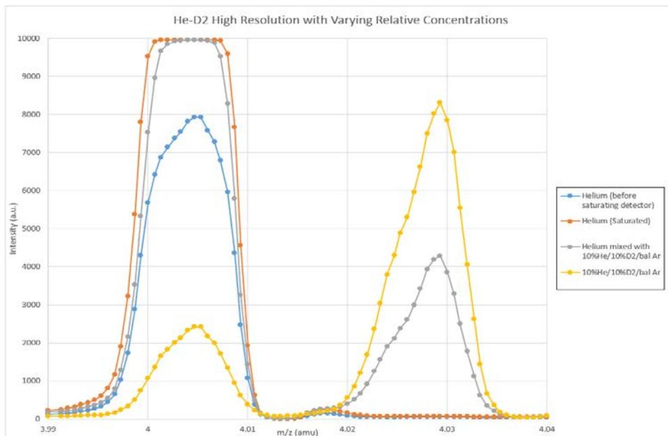
**Figure 8.** High Resolution Scans of Varying Relative Concentrations of Helium and Deuterium Collected Using a One Second Scan Time, with 1500 Points/amu.
