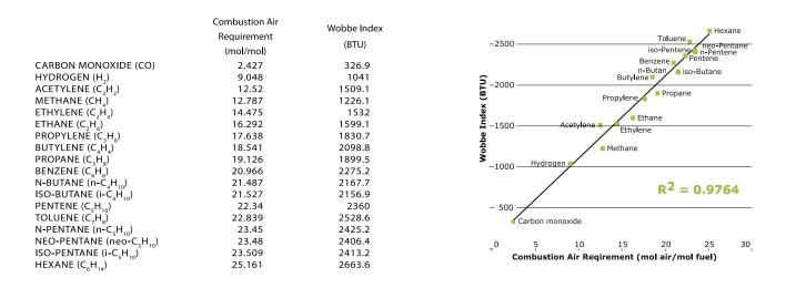
The table and graph above show the relationship of Wobbe Index and the Stochiometric Dry Air Requirement for some typical gas constituents. The correlation is close to linear ( $R^2$  = 0.9764) with an intercept close to zero. The residual oxygen method takes advantage of this correlation by linear extrapolation between measurements of known calibration gases.  $R^2$  for typical natural gas constituents plus hydrogen and CO is 0.9888.
