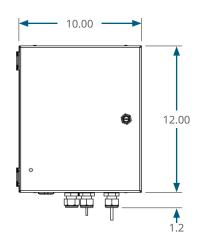
LAB 508 UV-VIS Dimensions – Bottom View
