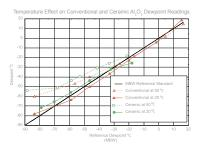
The temperature coefficients of conventional and ceramic sensors relative to their sensitivity are too large to allow for an accurate compensation through software.
