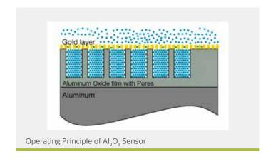
The advantages of the HTF sensor technology are a result of the proprietary manufacturing method in which the aluminum oxide layer is made to be hyper thin as well as extremely hygroscopic. This results in a very sensitive sensor with fast response.
