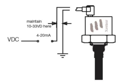
Operation with DC Power Supply Dew Point viewed on Instrument Display and available as Voltage output
