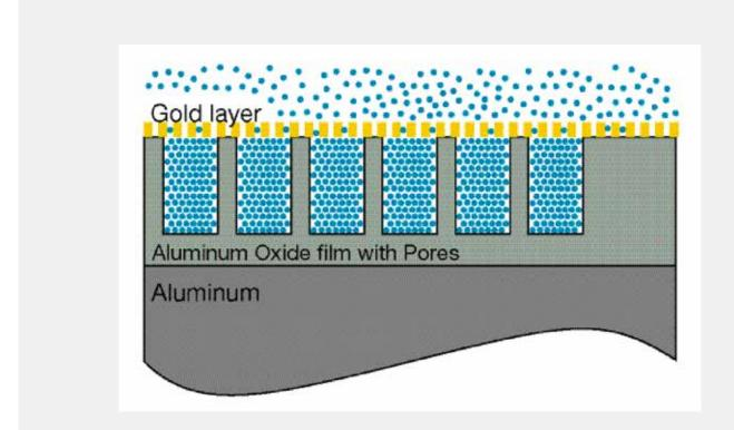
Operating Principle of Al<sub>2</sub>O<sub>3</sub> Sensor
