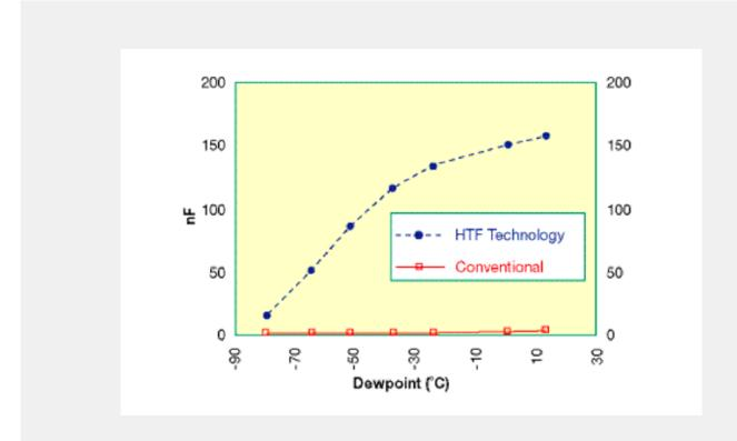
Hyper Thin Film vs. Conventional Al<sub>2</sub>O<sub>3</sub> Sensor. Change of Capacitance with Dew Point
