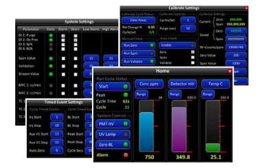
The GUI software also includes user setup and password security, as well as plotting of real-time analysis data and historical settings.
