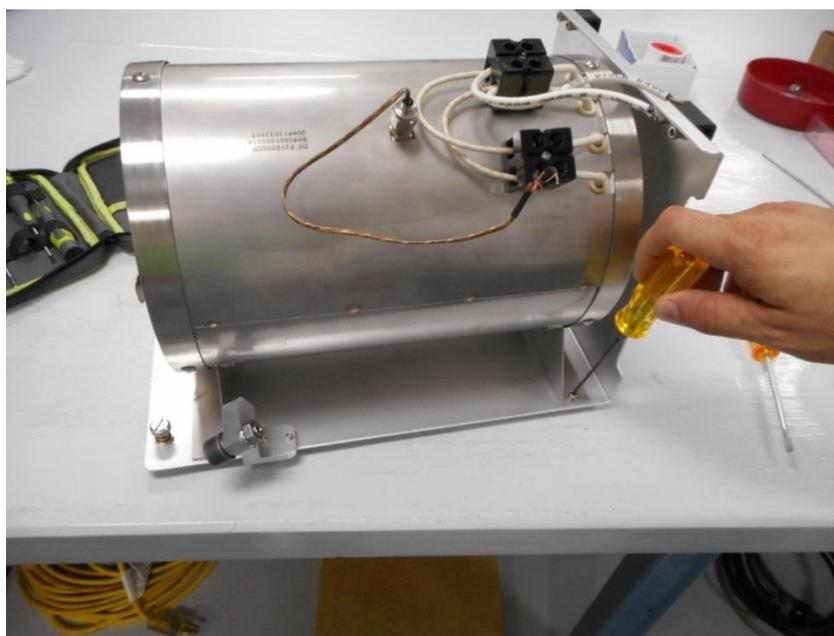
Remove all four furnace mount screws to complete the disassembly process
