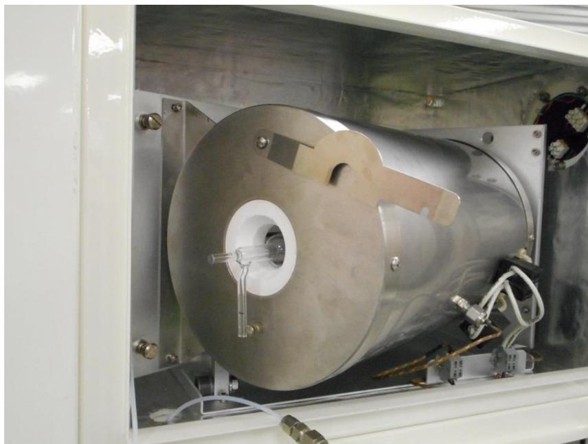
The combustion tube is now ready to be removed
