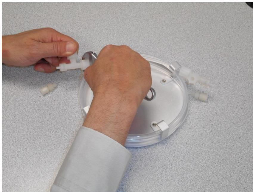
Next, loosen but do not remove the ¼" inch fitting on both ends
