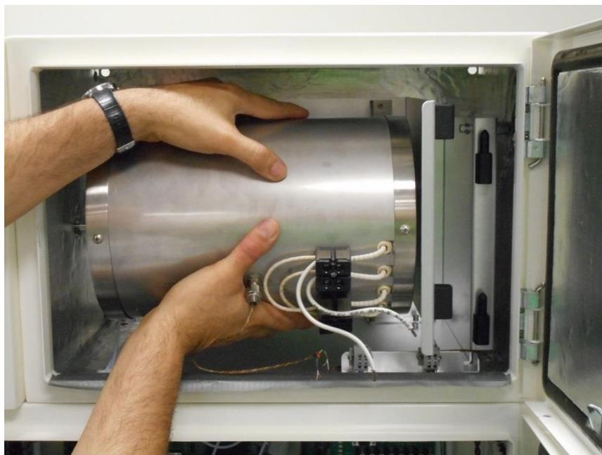
Carefully lift the furnace up off of the pin hinges and remove from the furnace chamber
