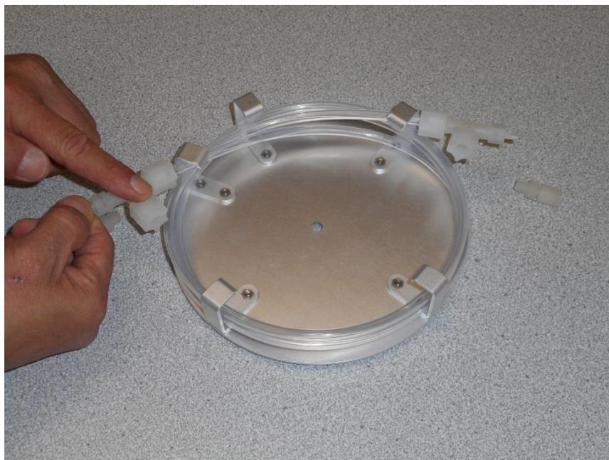
Holding the inner tube, rotate the T-fitting to point toward the inside on both ends
