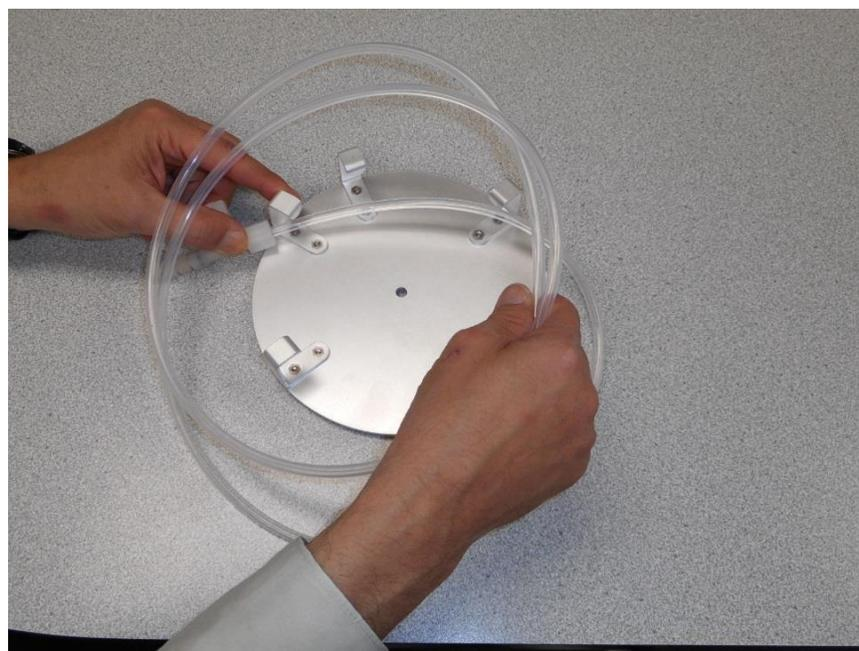
Begin by placing the tubing inside of the mounting bracket
