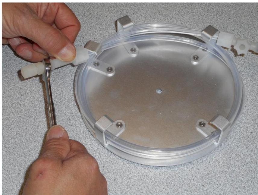
Using a 7/16" wrench, loosen and remove the 1/8" fittings on both ends
