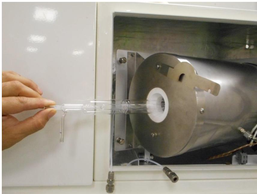
Carefully and slowly remove the combustion tube from the furnace
