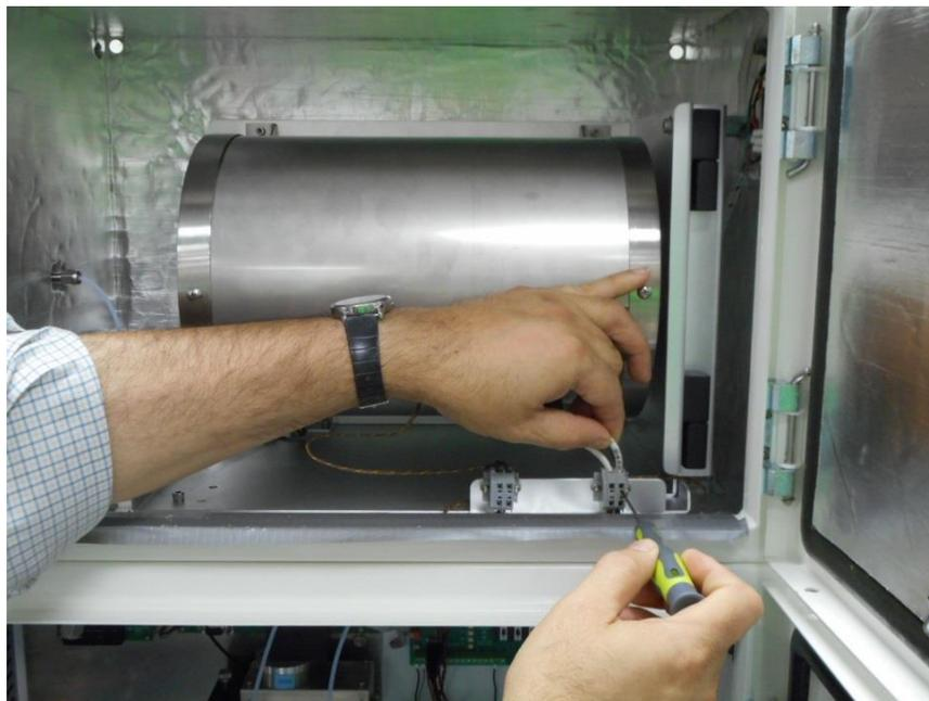
Using a small screwdriver to compress the terminal spring, remove both heater wires
