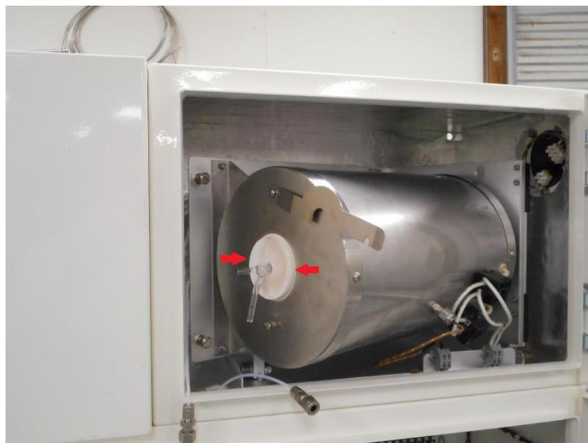
Carefully remove both ceramic insulators
