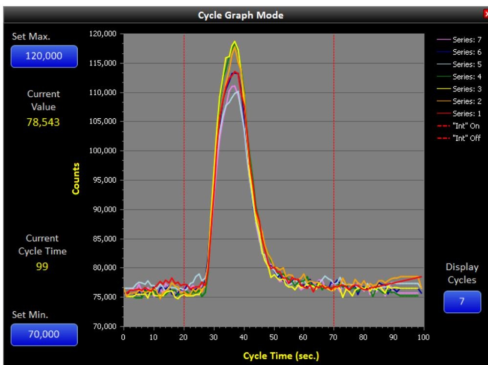
Figure 2.30 – Cycle Graph Displaying Multiple Trace Concentration Peaks
