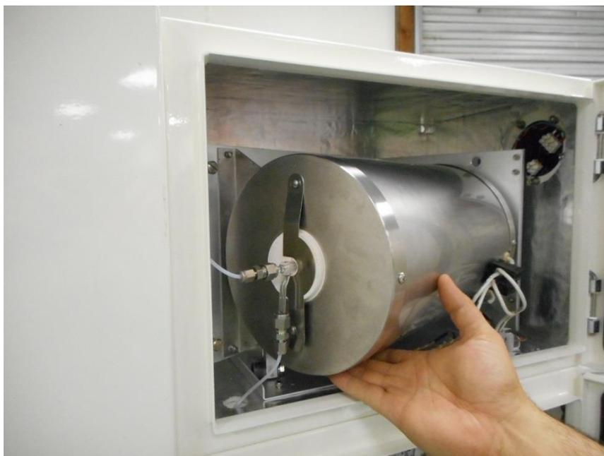
Gently swing the furnace outward. The furnace incorporates a special roller bearing for support and allows near effortless movement.
