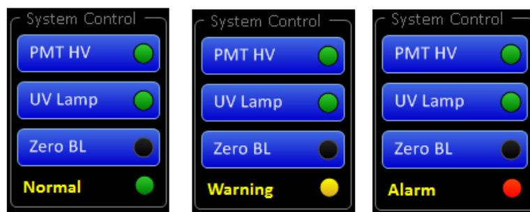
Figure 2.9 – Normal, Alarm, and Warning Status
