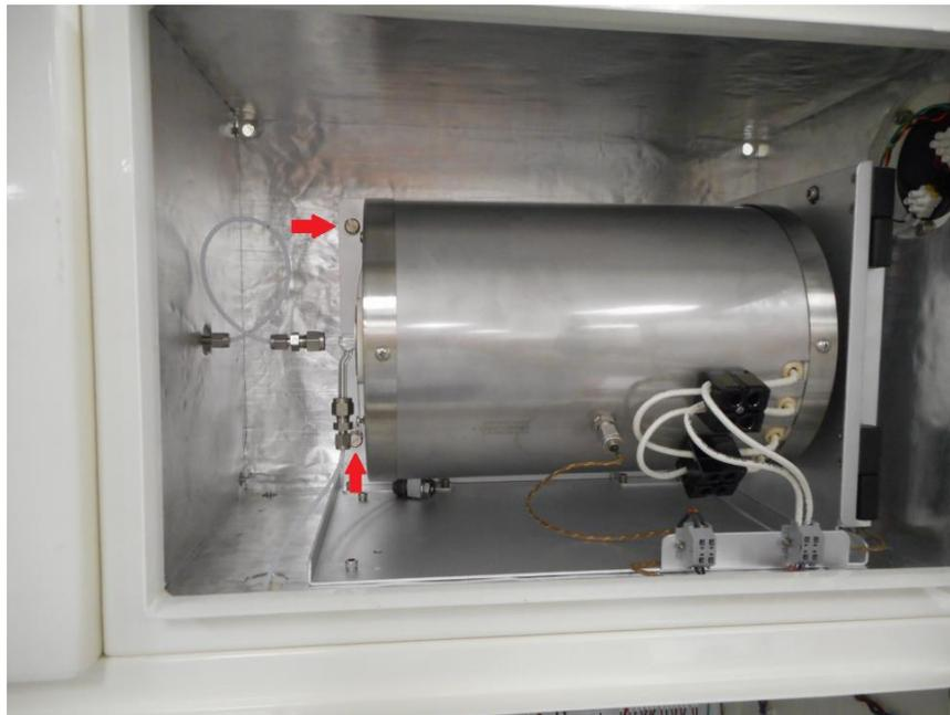
Begin by loosening the two screws indicated above inside the furnace chamber
