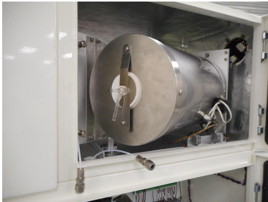
Fittings shown detached from combustion tube
