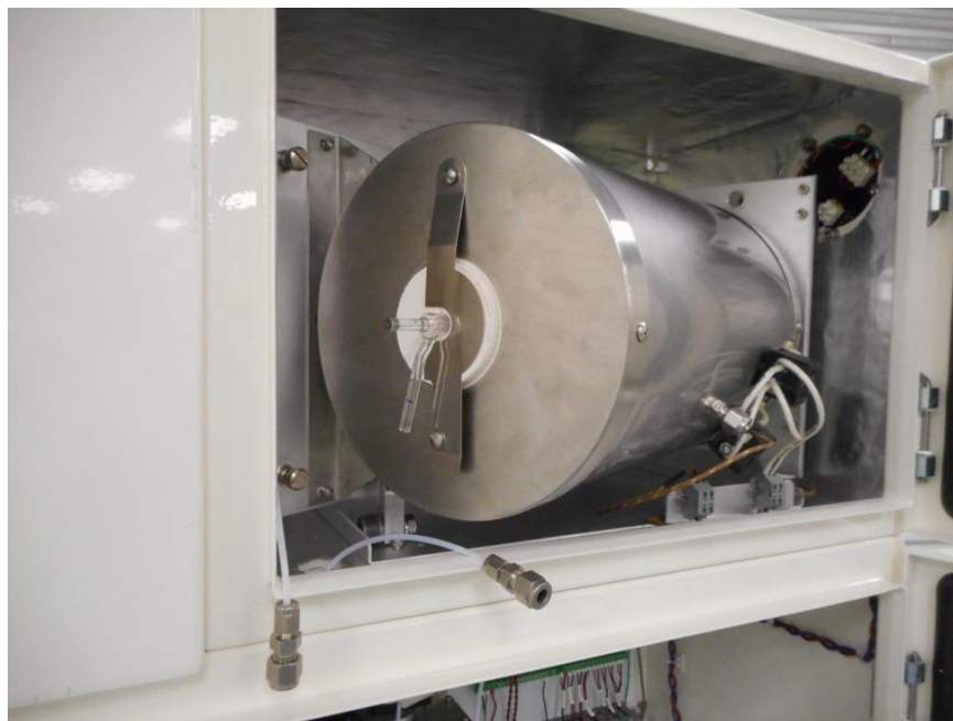
Fittings shown detached from combustion tube
