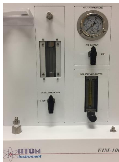
Figure 136 EIM with LPG Sightglass and Gas Capability
