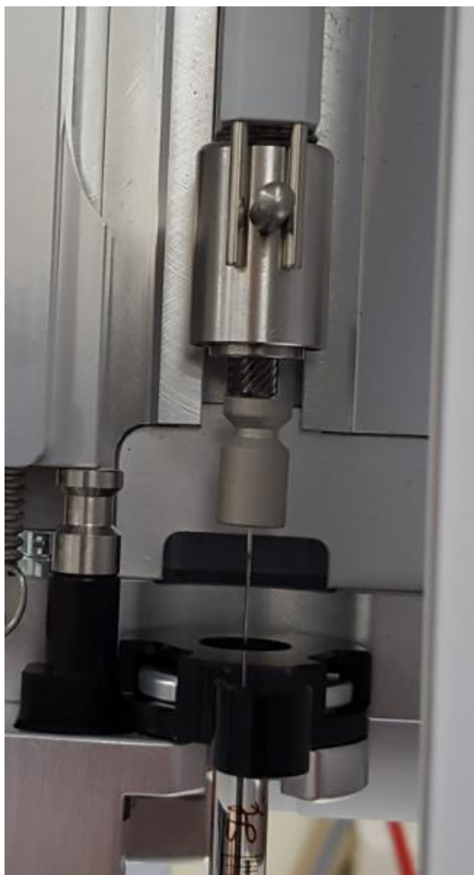
Figure 157 Plunger Released from Holder
