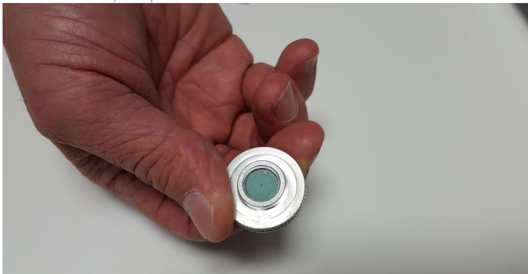
Figure 147 New Septum in Retainer Nut
