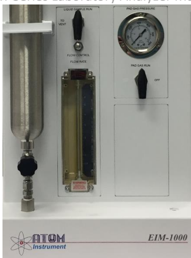
Figure 135 EIM with LPG Flowmeter
