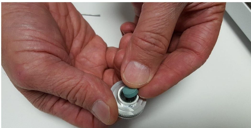
Figure 146 Used Septum out of Retainer Nut
