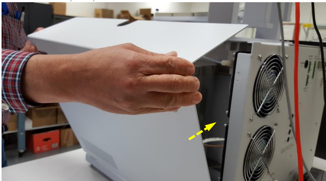
Figure 149 Reinstalling of Side Panel
