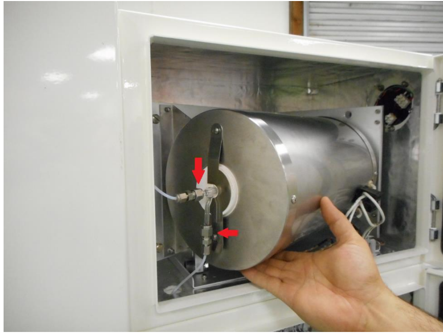
Loosen and detach combustion tube inlet and outlet fittings
