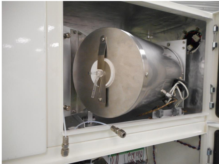
Fittings shown detached from combustion tube
