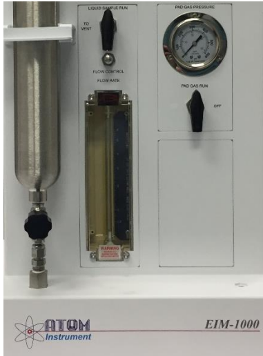
Figure 135 EIM with LPG Flowmeter
