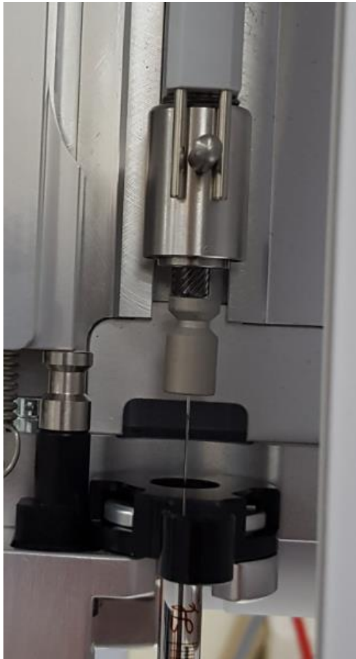
Figure 157 Plunger Released from Holder
