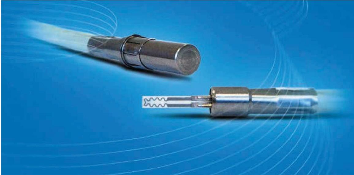
The heated electrolyte has an initial voltage ( $U_0$  approximately zero mV) in the absence of combustible gases (H<sub>2</sub>, CO or CH<sub>4</sub> or C<sub>3</sub>H<sub>8</sub>, etc). In presence of these gases, the output voltage increases (see chart below) as these gases are oxidized at the hot surface of sensor
