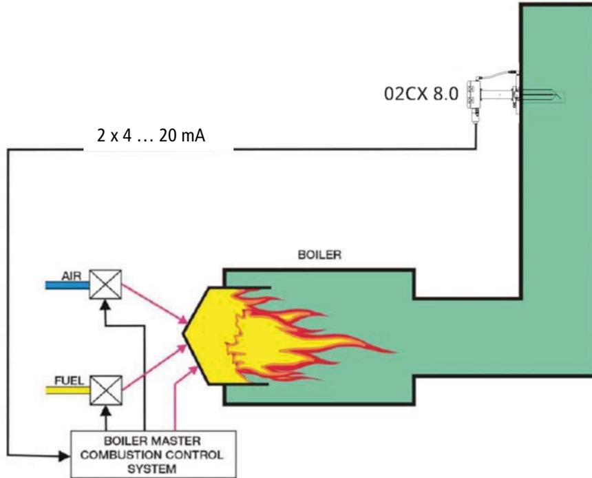
Optimum combustion conditions are achieved by decreasing the amount of excess air in the stack gas to the point where combustibles start to increase. See combustion diagram below:
