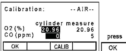
Second calibration shall be the span calibration with "GAS"
