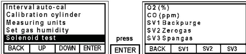
A manual switch ON or OFF of all 3 individual solenoid valves is possible.
