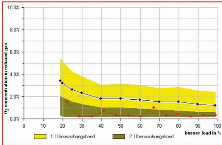
The difference between the yellow area and the brown area represents the degree of combustion optimization, which in turn represents savings in fuel.
