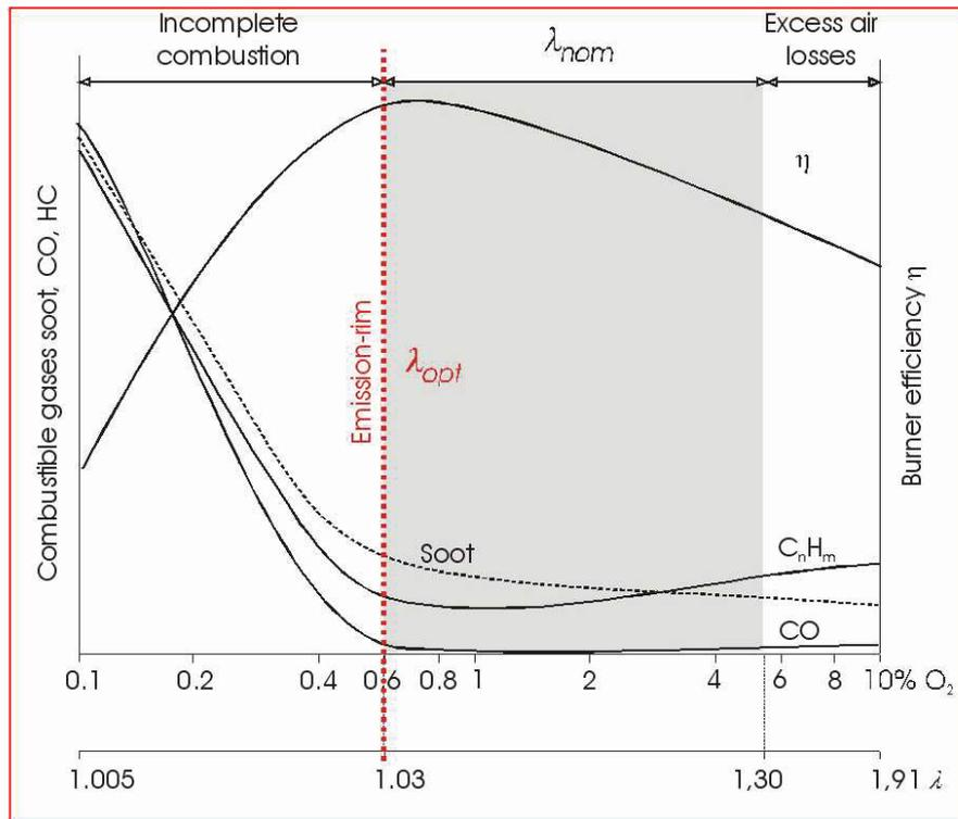
The absolute value of combustibles in the stack gas of a burner depends very much on the design and construction of the burner/boiler. Combustibles (CxHy) are lower in a well-designed system than they are one that is poorly designed.
