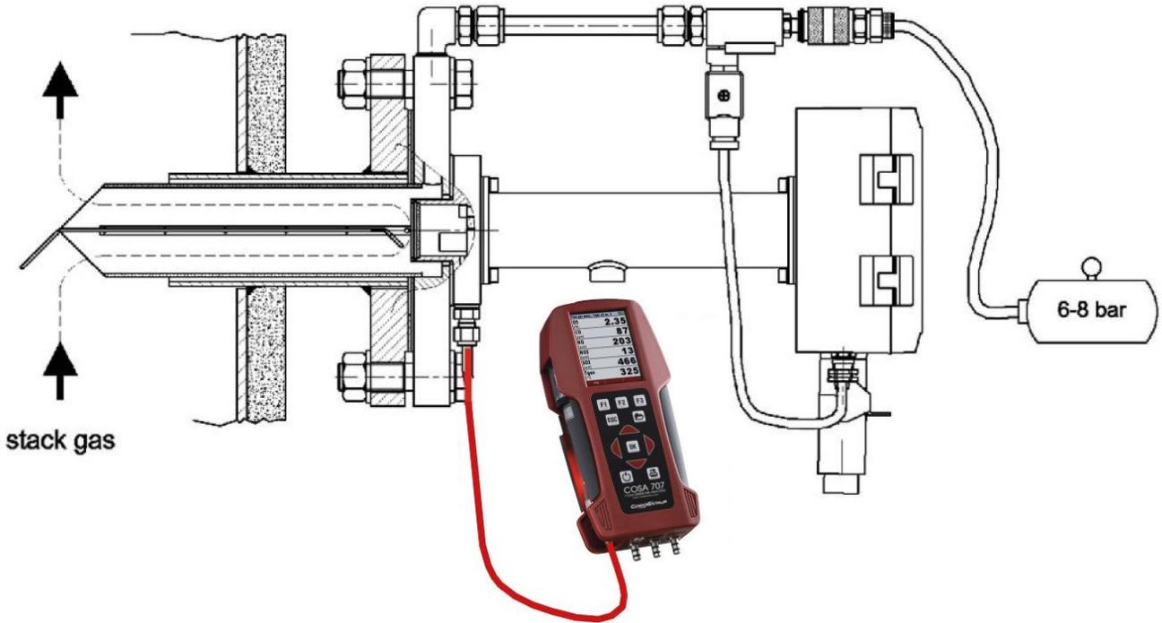
Use a portable analyzer to measure CO in the flue gas and to adjust accordingly the "desired value".
