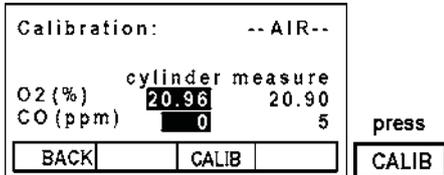
Wait approximately 5 minutes while instrument air is being supplied to sensors to allow signals to stabilize.
