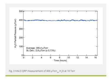
less. Figure 3 shows an example of a measurement of 400  $\mu$ Torr<sub>pp</sub> H<sub>2</sub>O at 10 Torr. At this level of H<sub>2</sub>O, the QRP operates significantly above its lower detection limit and yet way below its upper detection limit, which underscores the analyzer's
