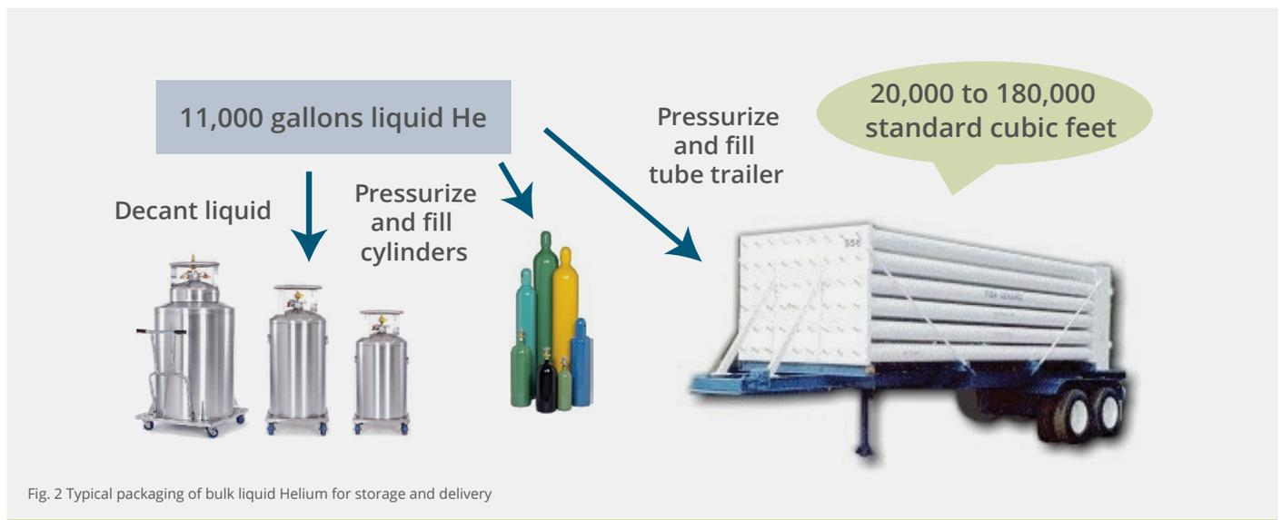
Typical Helium tube trailer filling operations perform several steps including gasification, compression, purification, and tube filling (schematically outlined in Figure 3). The goal is to fill the trailer tubes in the most energy and time-efficient manner possible, and there are several points where making a fast, accurate moisture measurement can assist in achieving this goal. The major monitoring points of interest are:
