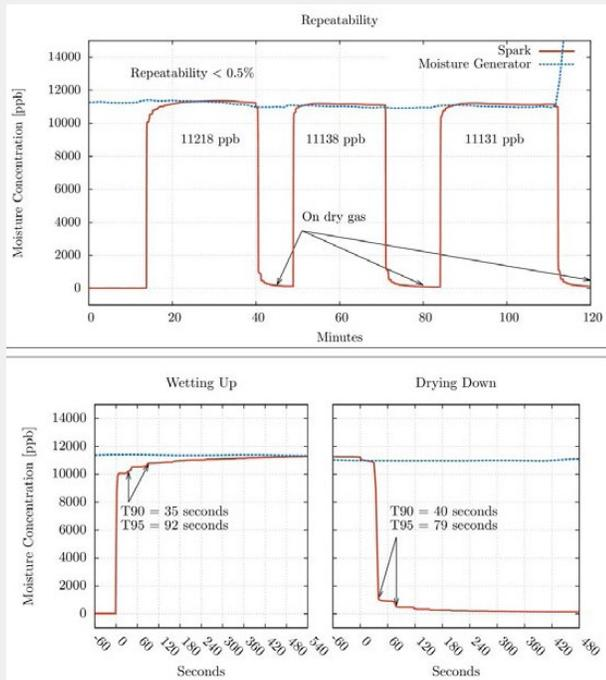
Fig. 5 Repeatability and speed of response of the Spark H<sub>2</sub>O
