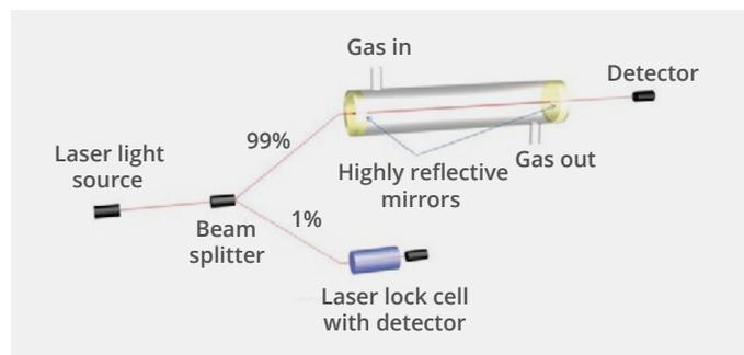
Fig. 6 Principle of Cavity Ring-Down Spectroscopy
