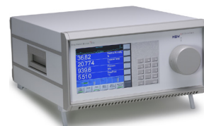
Chilled Mirror Hygrometers measuring moisture and humidity for reference and validation MODEL 373™
