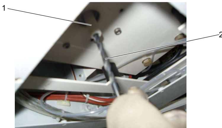
Fig. 101: Manual cleaning of the reactor pipe with a drill bit
