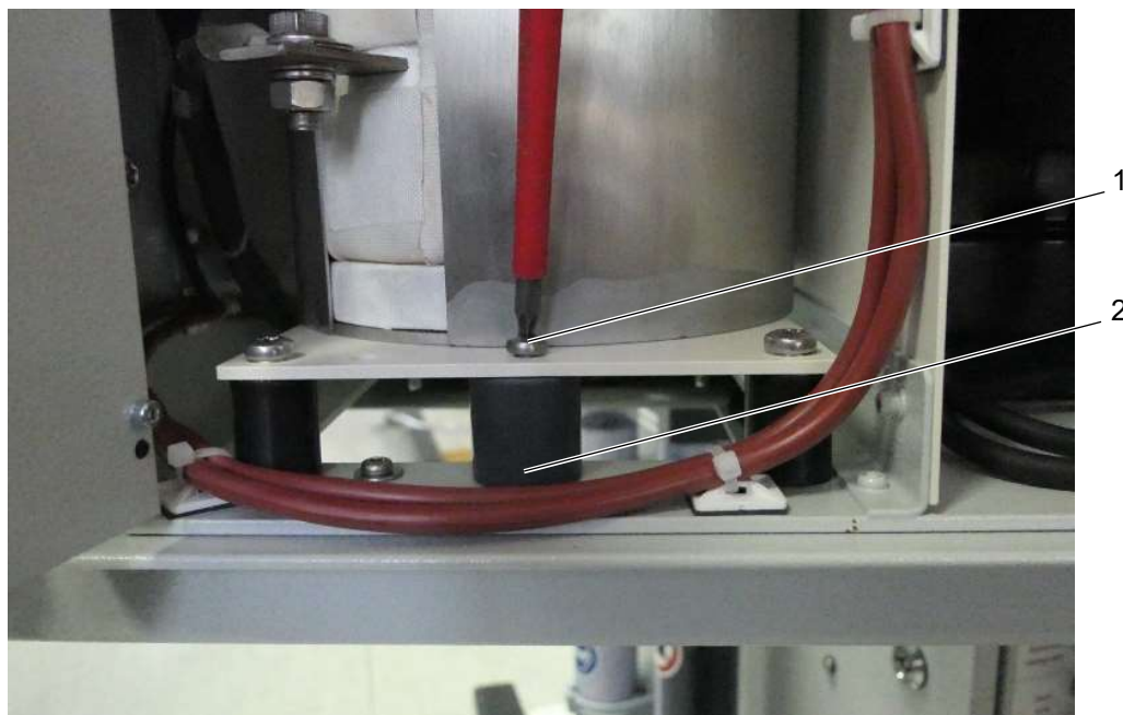
Fig. 37: Removing the transport locks of the furnace
