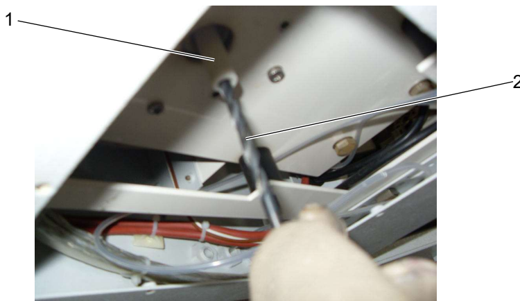
Fig. 88: Manual cleaning of the reactor pipe with a drill bit
