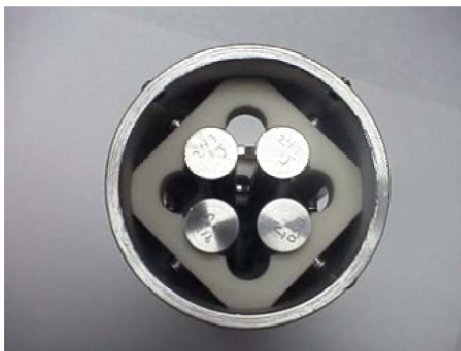
Figure 1. End view of 8.5 mm diameter rod quadrupole mass filter.
