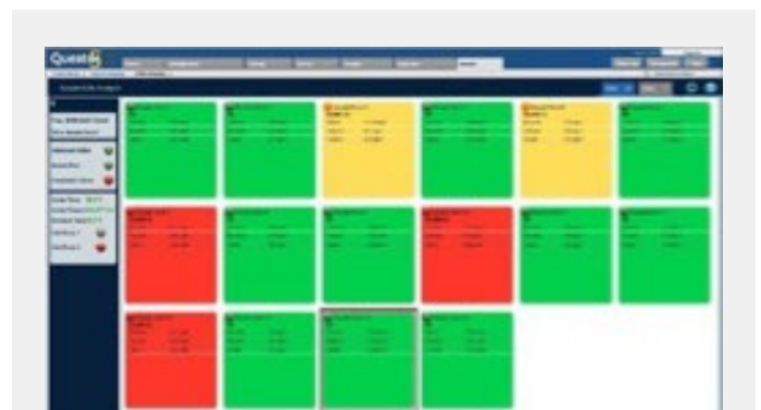
Figure 4: Questor5 software user interface showing Level 1 (yellow) and Level 2 (red) alarms.
